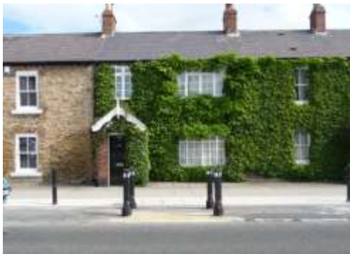
Plastic bollards and buff tactile paving are modern interventions that can sit uncomfortably within an otherwise traditional setting.
