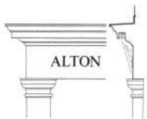
Discreet strip lighting concealed underneath the cornice.
