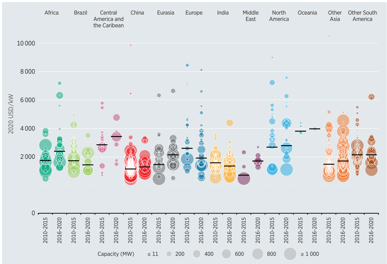
Figure 6.5 Total installed cost by project and capacity weighted averages for large hydropower projects by country/region, 2010-2020
