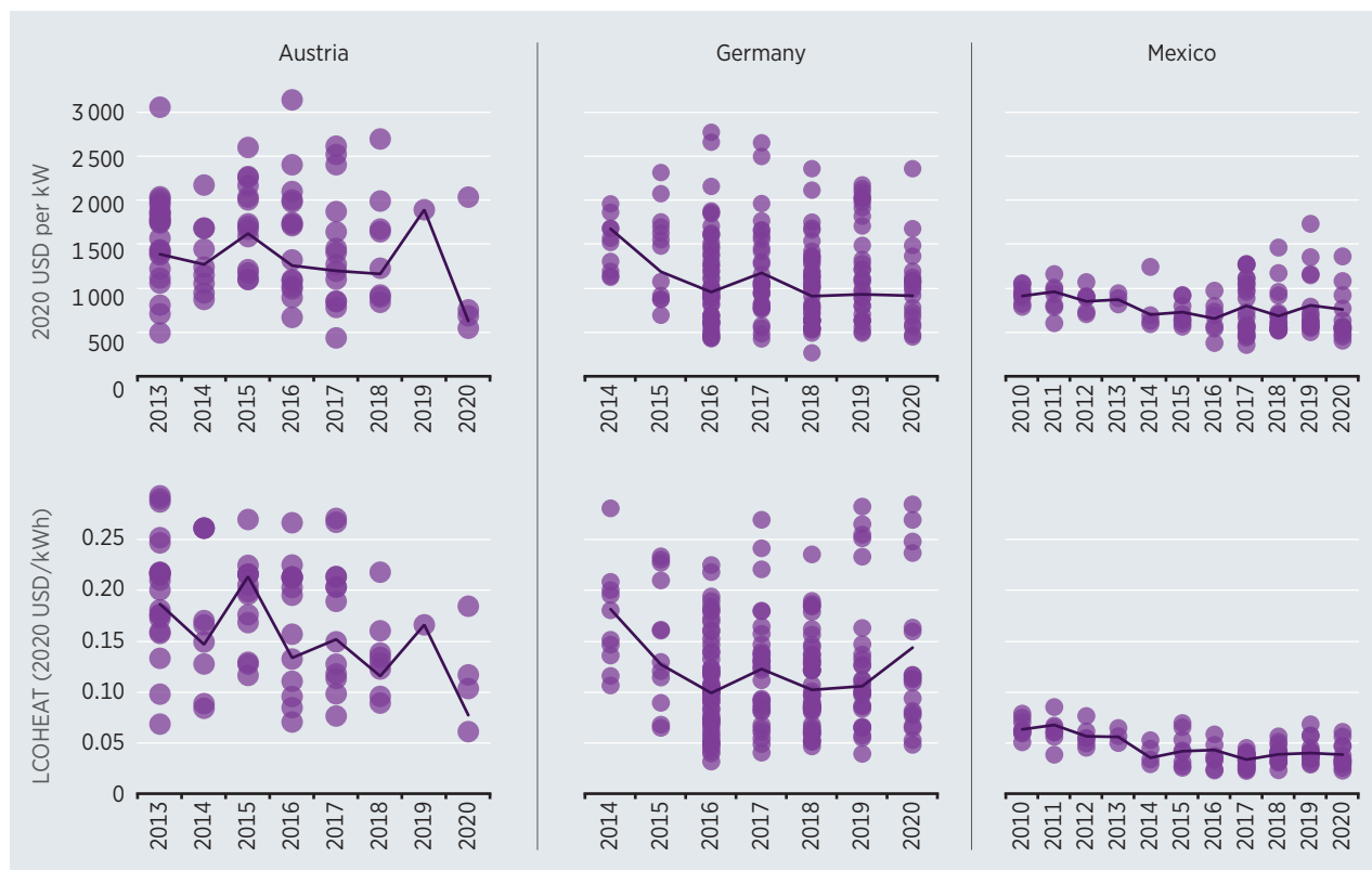
Figure 9.2 Total installed costs and LCOHEAT for commercial and industrial-scale solar thermal plants in Austria, Germany and Mexico, 2010-2020
