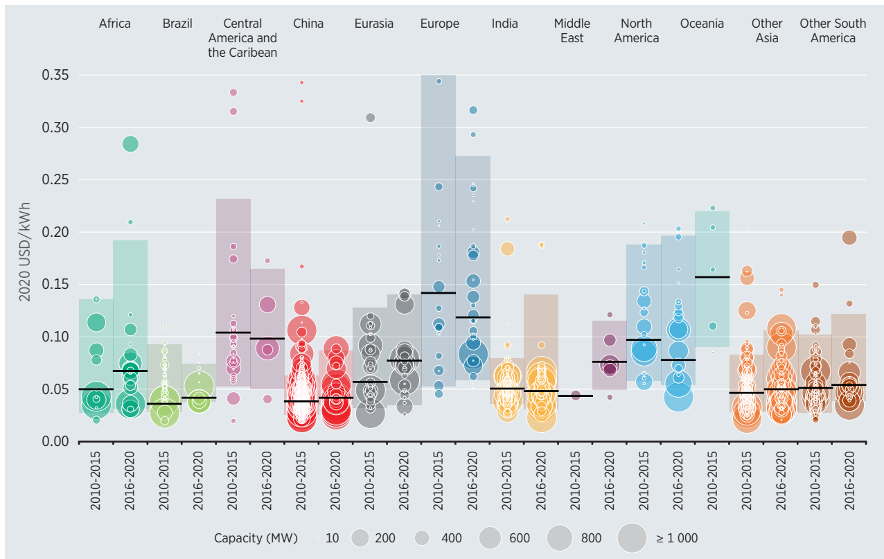
Figure 6.7 Large hydropower project LCOE and capacity weighted averages by country/region, 2010-2020
