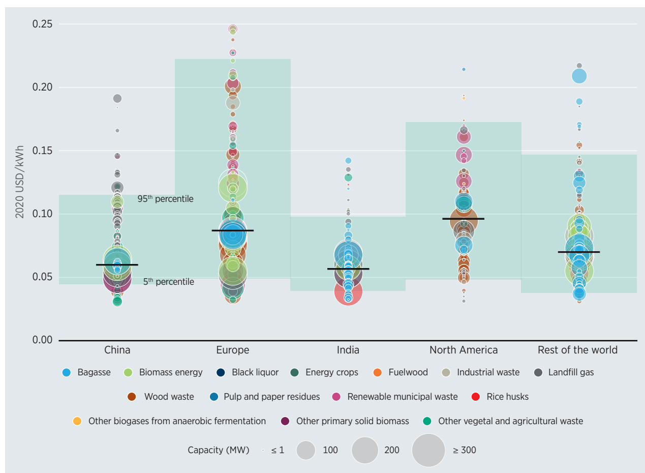
Figure 8.5 LCOE by project and weighted averages of bioenergy power generation projects by feedstock and country/region, 2010-2020
